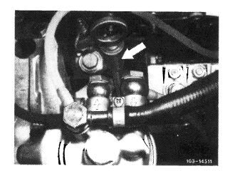
Oil dipstick tube with oil removal connection
